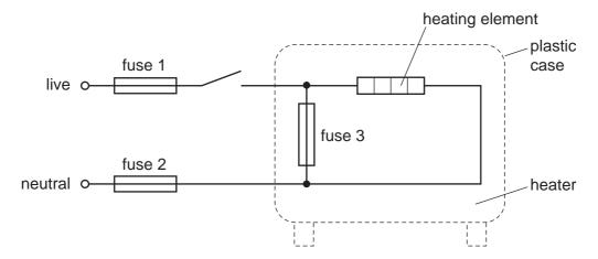
Which of the fuses are correctly placed?
